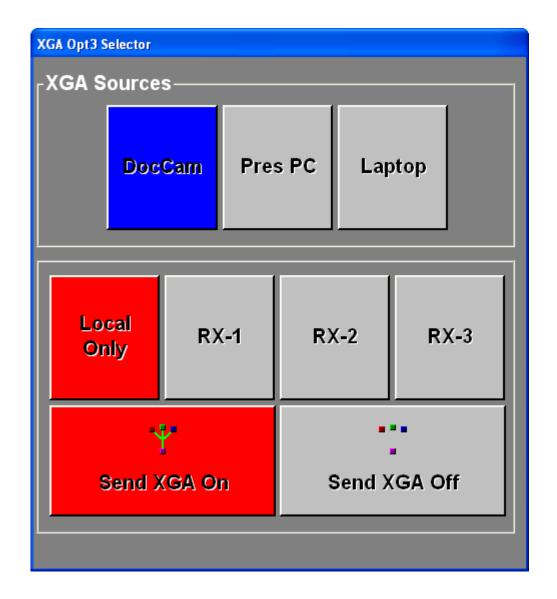
To return to the Originating Sites XGA, simply press the "RX-1" button at all remote sites. "Send XGA On" will automatically be turned off when one of the RX-1, RX-2 or RX-3 buttons are pressed. Finally, the Originating site must press the Local Only button to return to their XGA Sources. From here, selecting any XGA Source will again automatically transmit the High Resolution video to all remote sites in the session.
