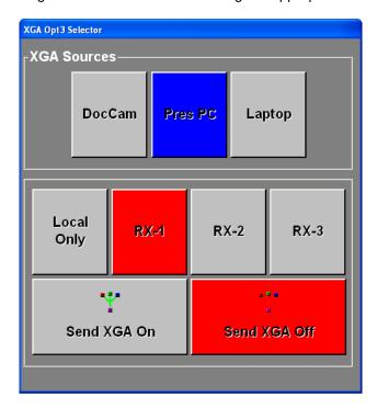
"RX-1" refers to Receive, or Incoming Video 1, while "RX-2" refers to Incoming Video 2, etc. In a quad monitor configuration, the Codecs, or Receive video signals, are positioned as such:
