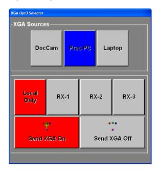
When the "Send XGA On" button is red, all remote sites will now be sent the high-resolution image of the selected XGA Source. You may select any composite video source from the DL-Navigator Program Sources at any time without effecting the XGA transmission (See Below).
