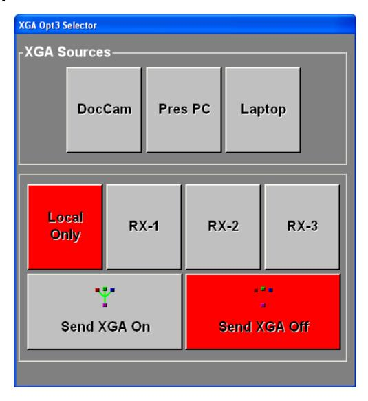
Above is the XGA Selector Control Form. This is where all High Resolution media sharing is controlled between sites when the XGA Option is installed. The following paragraphs describe how to operate the XGA OPTION-3 Sharing.
